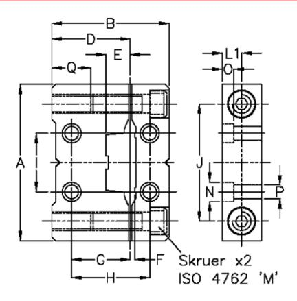
$$\begin{array}{lll} A & = 170 & I = 95 & Weight kg/1000 = 1.05 \\ B & = 100 & J = 140 \\ D & = 62.5 & L1 = 12.5 \\ E & = 19.5 & M = M12x50 \\ F & = 4.0 & N = 17.0 \\ For slide = NL 120 & O = 11 \\ G & = 35 & P = 11 \\ H & = 54 & Q = 35 \end{array}$$
